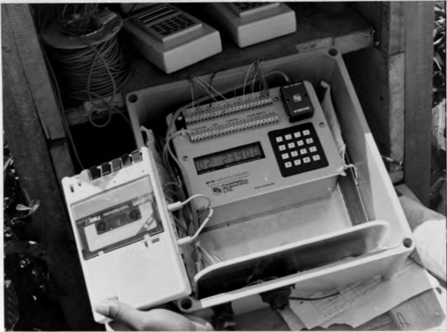
PLATE 2: Close-up of 21X Micro-logger showing thermistors connected to the channels. (Note the reading from one of the thermistors showing the air temperature).
