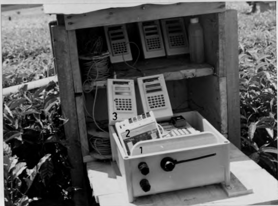
PLATE 1: (1) The 21X Micro-logger (Campbell Scientific Ltd. USA), (2) An ordinary cassette recorder and (3) the Millivolt integrators recording radiation, soil, air and plant tissue temperatures and saturated vapour pressure deficits of the atmosphere.
