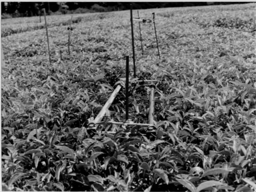
PLATE 3: Tube solarimeters measuring (1) Reflected radiation and (2) Total intercepted incident radiation and filtered incident radiation ( 0.7 \mu\text{m} to 2.5 \mu\text{m} ) to give PAR ( 0.4 - 0.7 \mu\text{m} ). Note: Total tube solarimeters are placed 30cm below the plucking table of each clone to measure maximum canopy extinction.
