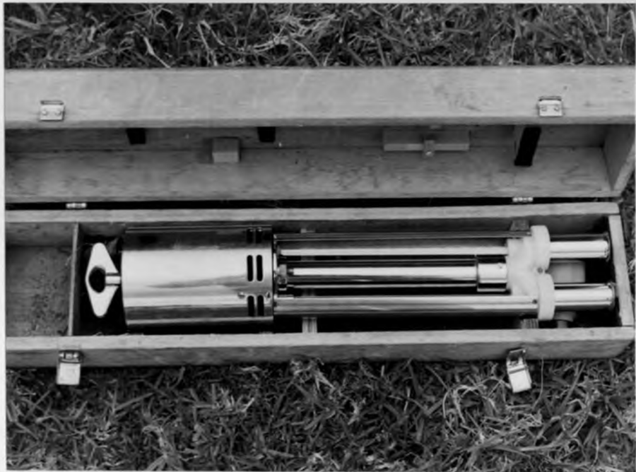
PLATE 5: A close-up of the Asman's Psychrometer showing the chambers holding the wet and dry bulb thermometers and the housing for the miniature fan on extreme right.
