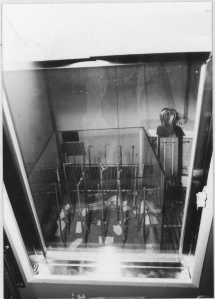
Fig. 5. An aquarium inside the climate chamber used in the laboratory experiments.
