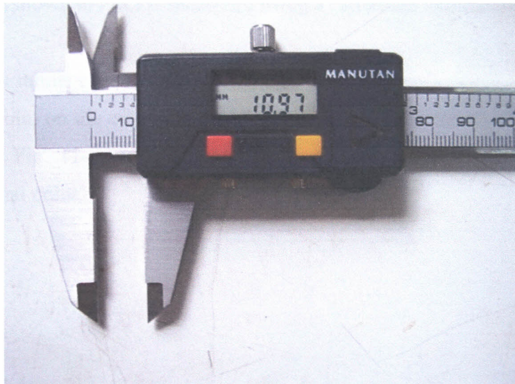
Fig.9. Showing the digital Vernier calipers used to take straight measurements
