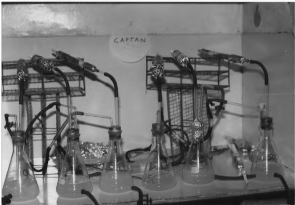
Figure: 6: Simple fermenters. Growth recorded at control (no captan) 10 and 50 ppm of captan. Observe clear YEM at 250 and 500 ppm of captan
