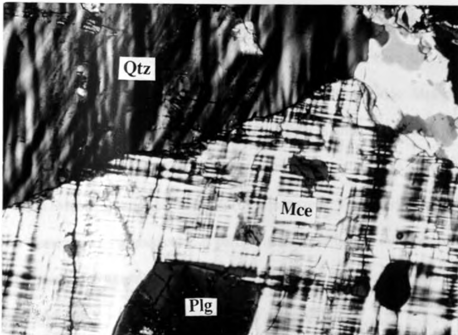
Plate 2.13 Photomicrograph of microcline (Mce) porphyroblast with exsolved plagioclase (Plg) and in contact with quartz (Qtz). Porphyritic granite (MU-29), Crossed polars, X 50.
