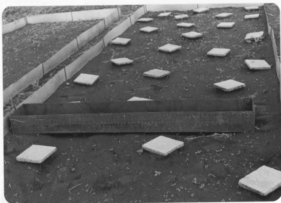
Plate 4. The trough used to supply water uniformly as overland flow (Photo was taken after the experiment was completed)
