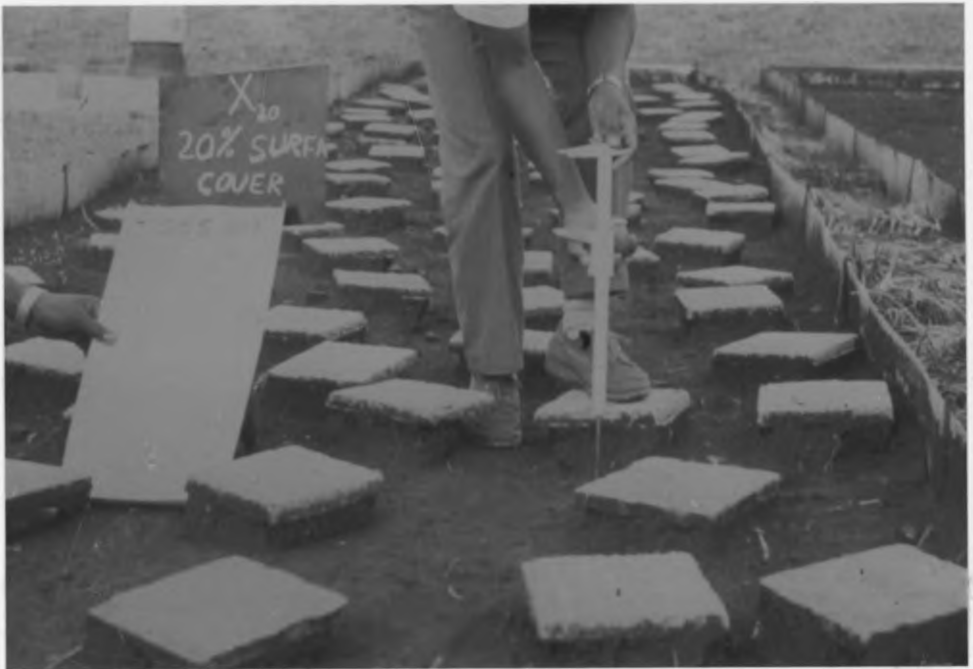
Plate 7. Measurement of the soil depth removed by the long rains
