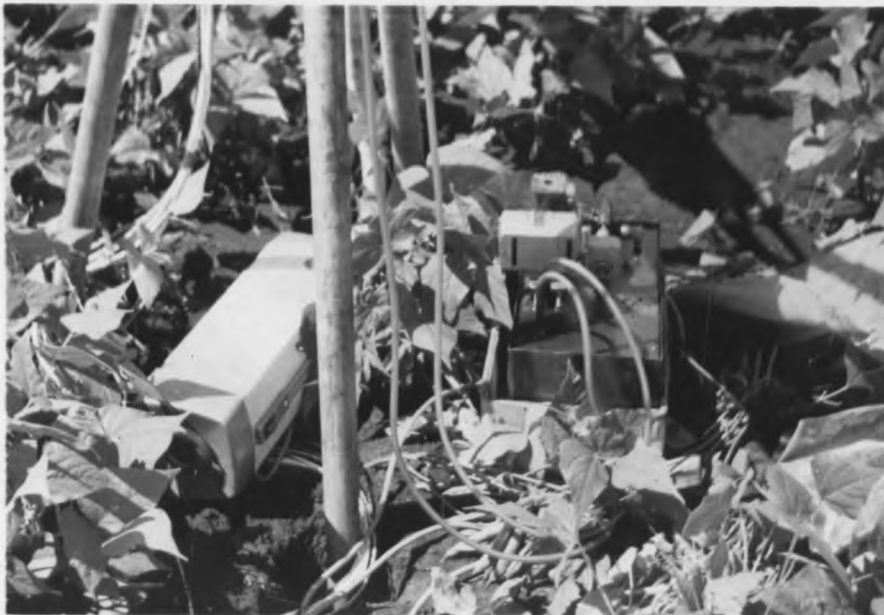
Fig. 20 : Operation of Bowen's Ratio equipment. (a) rotating boom above bean crop, (b) details of tripod support, vacuum cleaner for sucking air, and hydraulic system for rotating boom.
