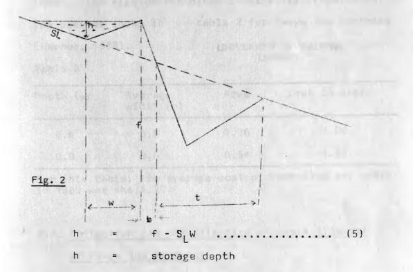
In the same publication, Larson discusses Grassed Backslope Terrace where excavation is done above the ridge in addition to that below the ridge to make the desired storage depth. In this project the formula developed by Thomas et al (1980) has been used to calculate storage depth and the volume of soil to be cut per 1 metre length of the ditch.
