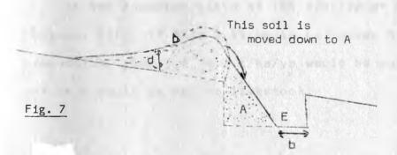
In this design, the soil is thrown up and pulled down again because this requires less skill compared to cutting the slope to the correct angle at the start.
