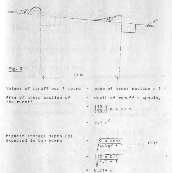
This equation was developed by Thomas et al (1980) on the assumption that the upper side of the ridge meets the land slope at 45°.
