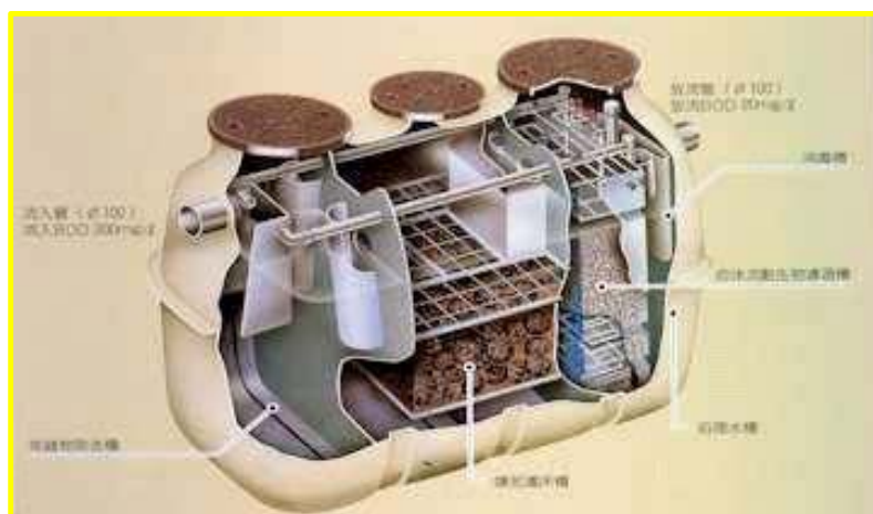
Figure 3: Gappei -shori johkaso that accept urine and feces, and grey water to treat and discharge in a neighbor water channel. (Source: Year 2001 Japan Waste Treatment Report, MoE, March 2004).
