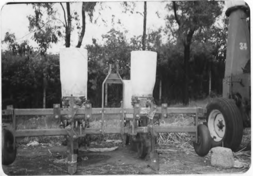
Plate 3 Conventional maize planter used for no-tillage planting
