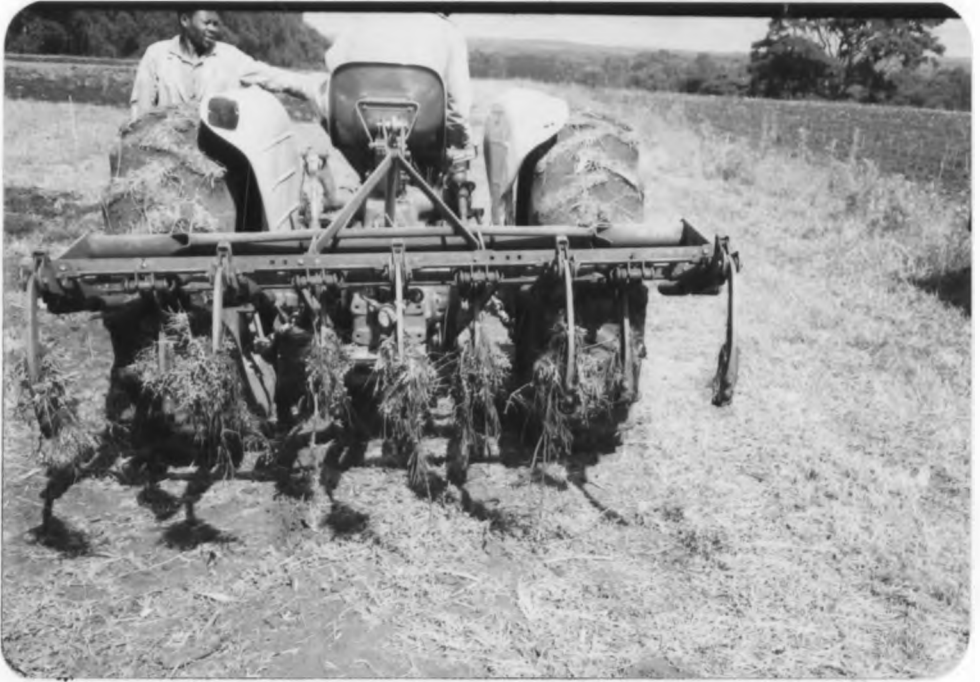
Plate 5 Tined harrow used for minimum tillage plots
