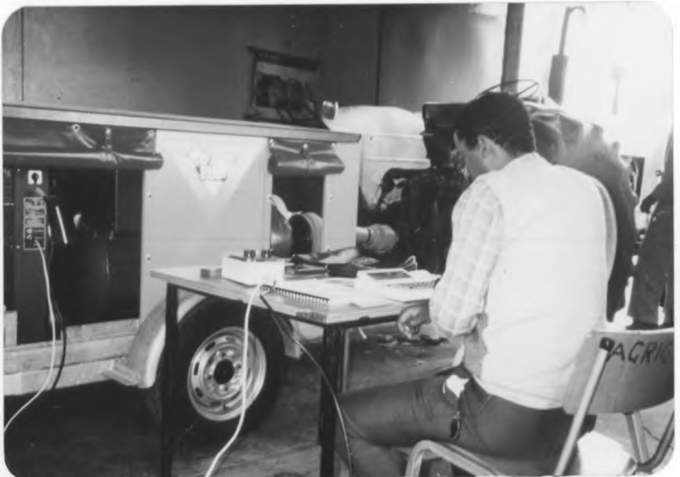
Plate 13 The Froment Dynamometer used to test the tractor PTO power
