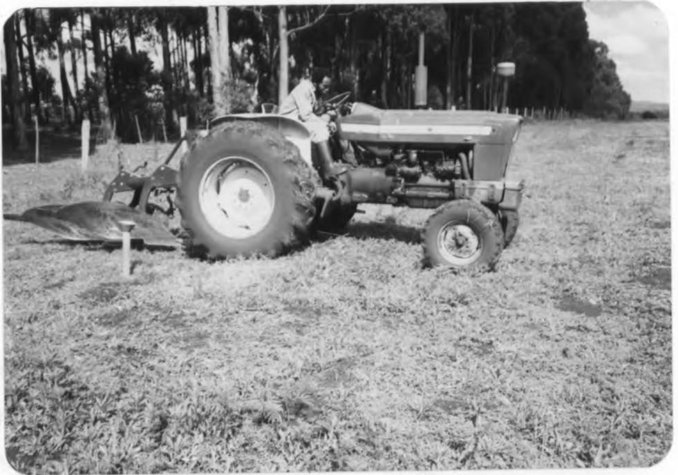
Plate 7 The two bottom mouldboard plough used for the conventional tillage treatments
