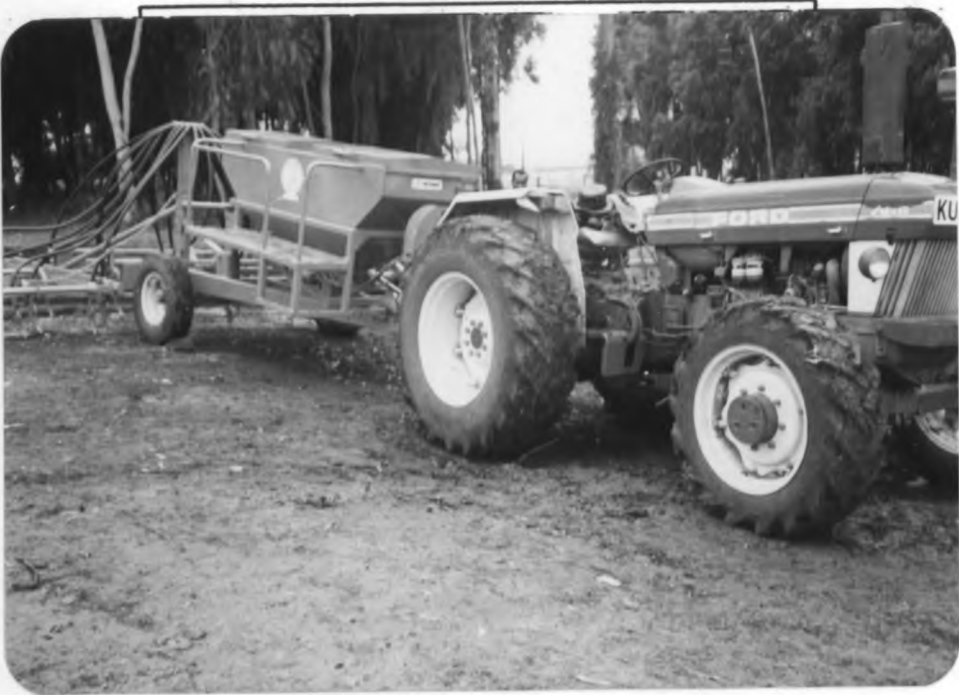
Plate 1 The Ndume air seeder used for wheat no-tillage planting
