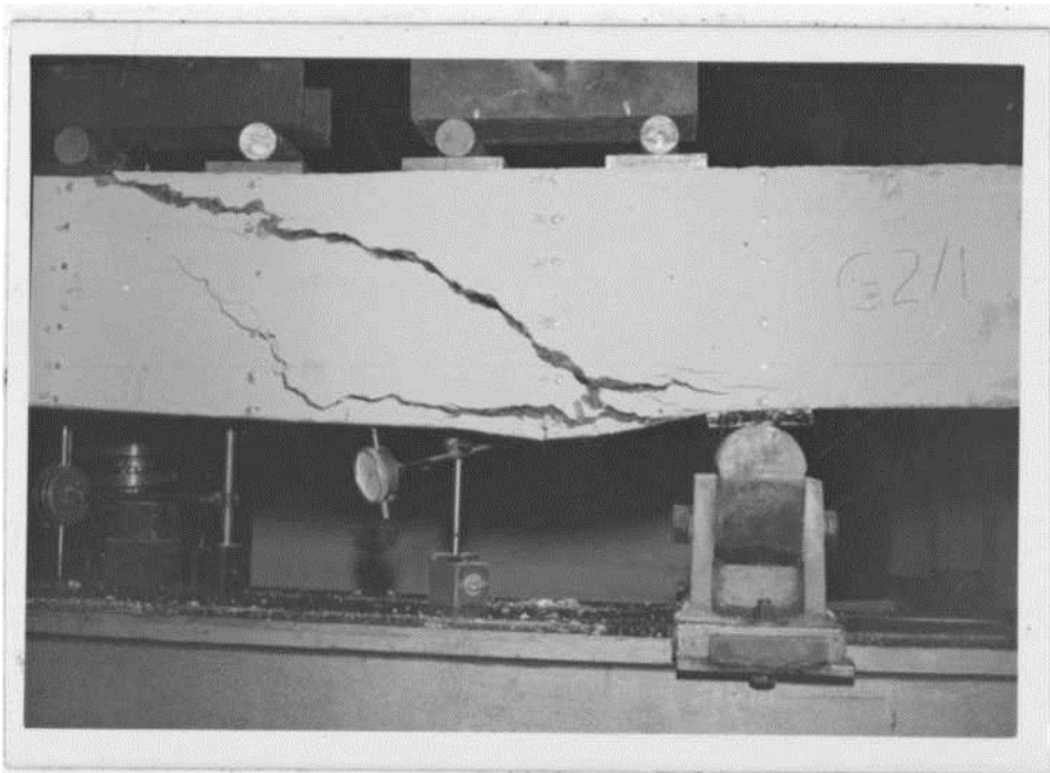
PLATE B6: Close-up of the failure diagonal crack of beam G2/1*
