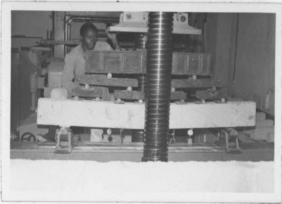
PLATE B 13: Diagonal cracking of beam G2/L during loading.
