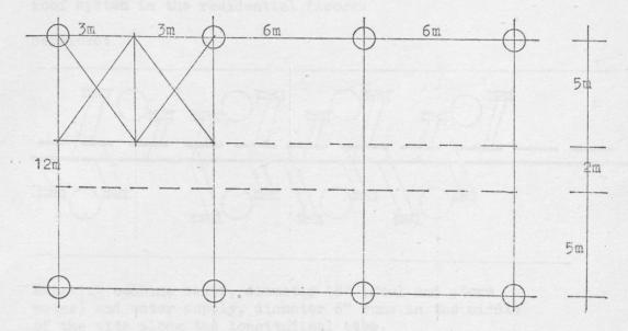
Structural system of 6m x 12m can accommodate the smallest office (3mx5m) on either with a corridor 2m wide. A range of office spaces can be fitted from that of 3m x 5m office to poor type areas of 6m x 12m or even 12m x 12m.
