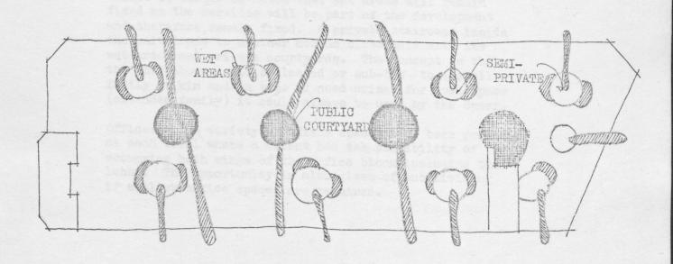
Horizontally circulation is partially exposed to urban environment with internal and external circulation on the first floor, while ramps are introduced for vertical circulation up to the second floor, being totally public.
