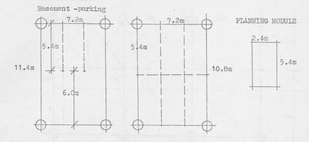
Structural grid of 7.2m x 11.4m allows a maximum of 3 car park with a 6m lane for turning and access.
