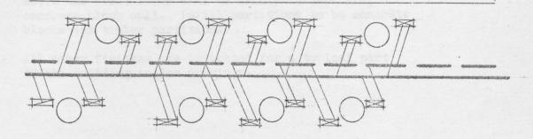
Existing combine sewer, diameter 18" (foul and storm water) and water supply, diameter 6" runs in the middle of the site along the longitudinal edge.
