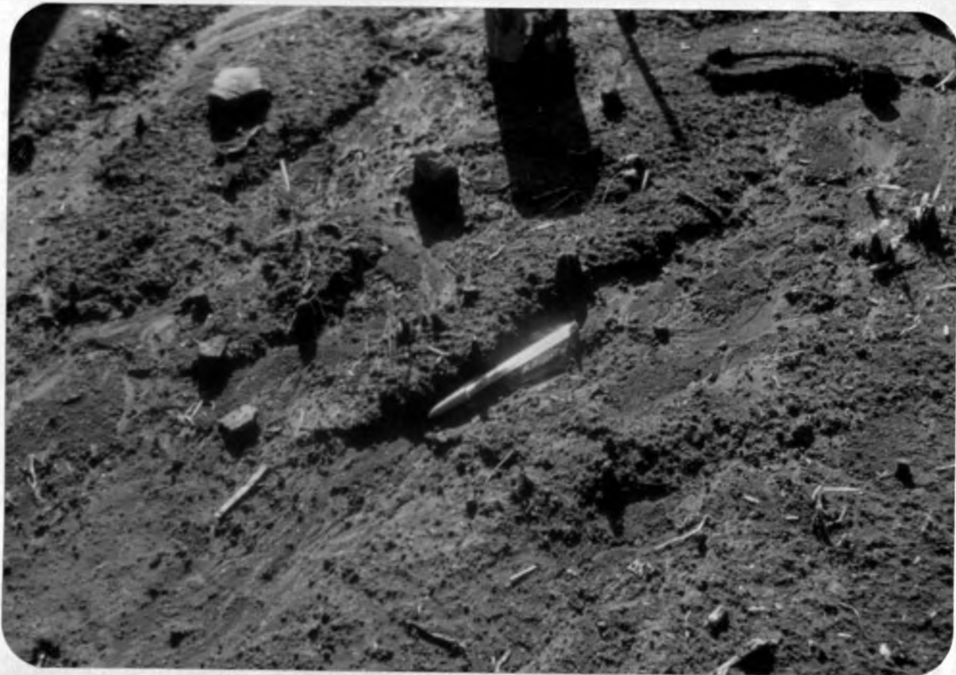
Plate 7. Picture showing surface condition after the wet run of 80 mm/hr simulated storm and effect of trash and gravel in protecting the soil.
