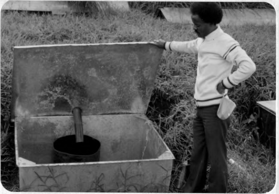
Plate 1. Storage tanks and conduit pipe used in the runoff plots
