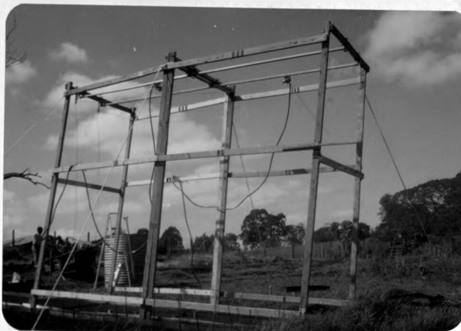
Plate 4. Rainfall simulator used to simulate 80 mm/hr storm
