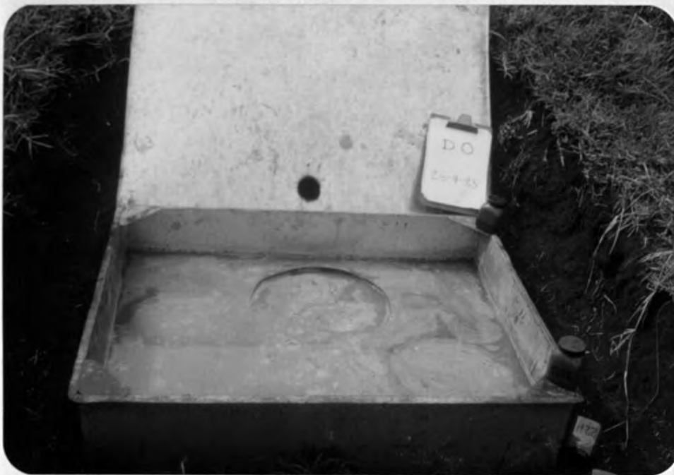
Plate 3. Runoff collected on 26/4/83 and the 0.54 l. sampling plastic bottles.
