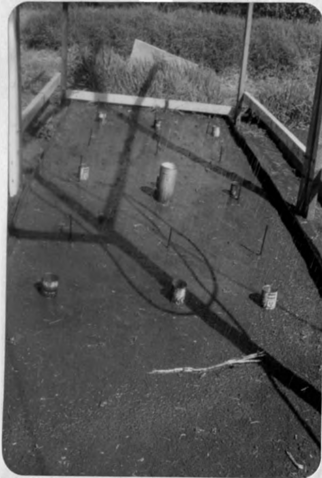
Plate 8. Picture showing uniformity of application of simulated storm (80 mm/hr) on plot D3.
