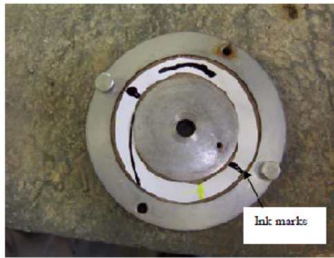
Figure 6. Ink-marks spread strategically and ready for the test
