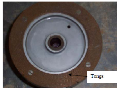
Figure 18. Upper platen of the ring shear detailing the tongs
