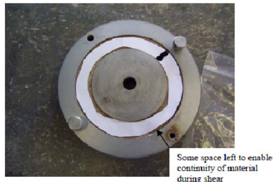
Figure 5. Annulus paper ring being fitted into the cell cavity
