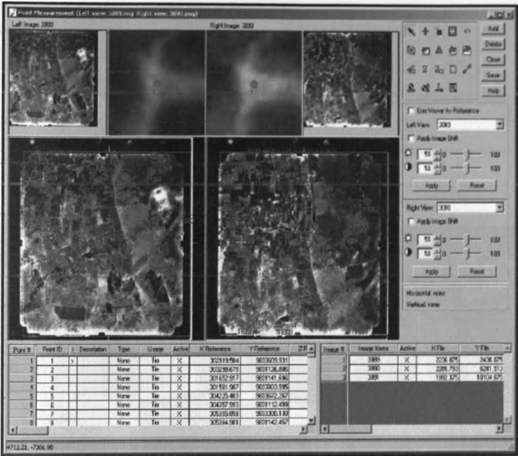
Figure 3.5: Automatic tie point measurement
