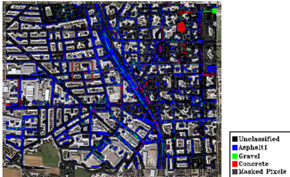
Figure 1: SAM classification using threshold of 0.08 (radians)
