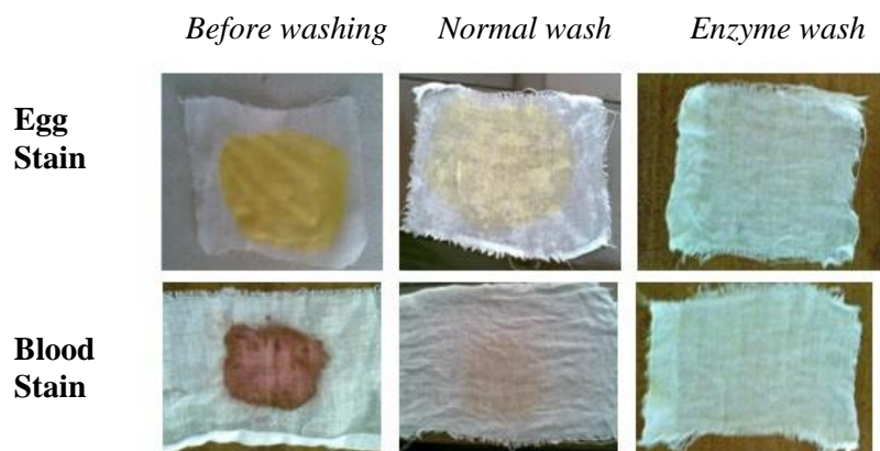
Fig. 6: Evaluation washing performance of protease R-11 using blood and egg stained cotton cloth.
