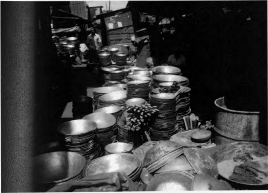
Figure 9: Karai's and shallow pans made from used oil drums whose paint is removed manually by gradually rubbing coarse sand and a rag.
