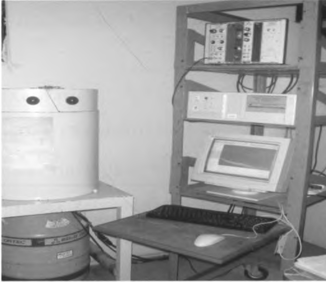
Fig 4.6 The gamma-ray spectrometer setup comprising the HPGe detector (inside the lead shield) and the associated electronics.
