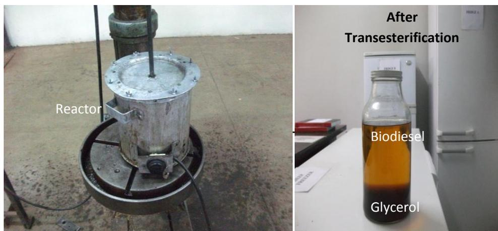
**Fig 3.5: Reactor during transesterification and separation of Biodiesel and Glycerol.**
