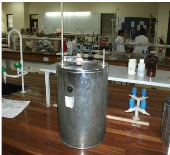
**Fig 3.8: Constant –volume bomb calorimeter**
