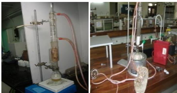
**Fig 3.4: Soxhlet apparatus for solvent extraction.**
