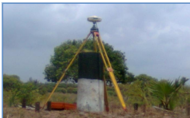
Fig 4.2 Leica GPS Receiver over control point SKP 201.S.1
