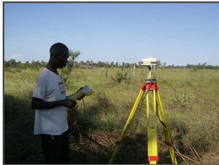
Fig 4.4 Leica GPS Satellite Receiver at control point SKP 200.S.10
