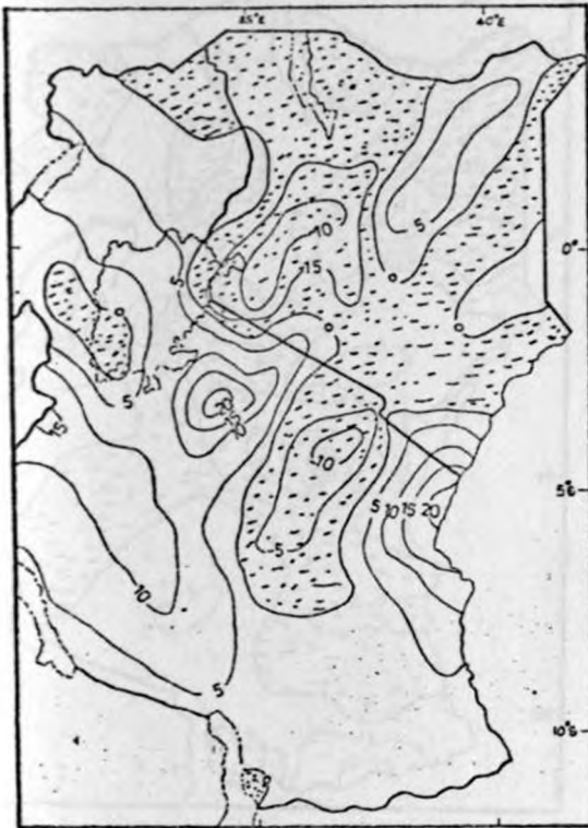
Fig. 30(b) : Mean divergence field ( \times 10^{-6} \text{ s}^{-1} ) at 3050 m AMSL in July.
