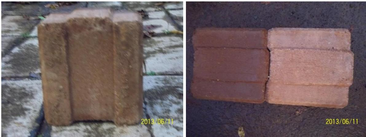
**Plate 5 & 6: Standard Hydraform Block (Sample of Interlocking Stabilised Soil Block)**
