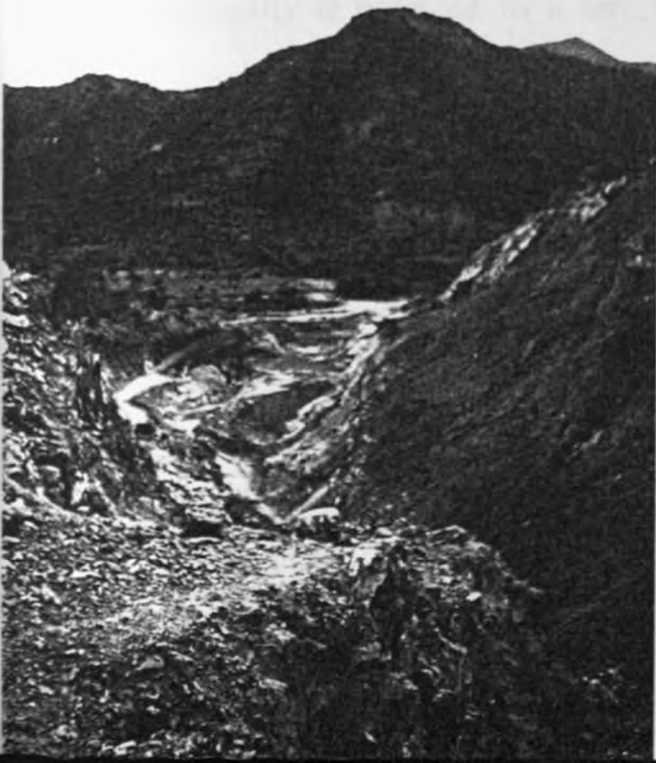
Plate 5.11 shows the depth of fluorite mineral extraction site. Note that water from fluorite bearing water table accumulates at the bottom of the pit.
