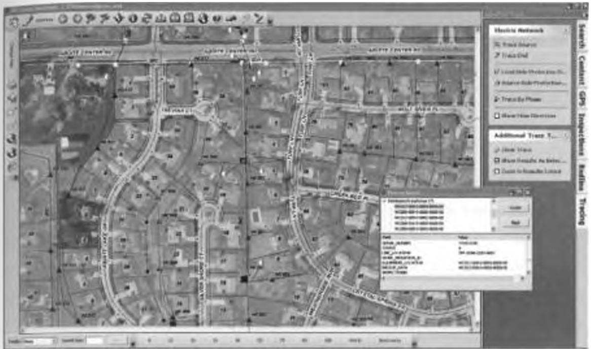
Figure 2.1 Color-coding facilities by their electrical phase and tracing functionality allows field personnel to quickly assess the severity of an outage.
