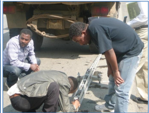
Figure 3-7 Adjusting the Benkelman in preparation for measurement
