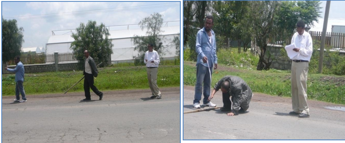
Figure 3-19 Visual estimation of cracking area Figure 3-18 Rut depth measurement
