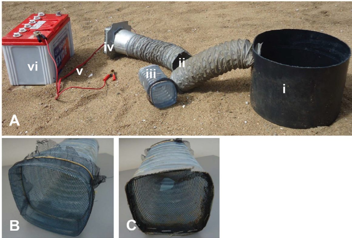
Figure 4. Ovi-ART gravid trap prototype. (A) Trap parts: i) round black bucket, ii) suction tube prepared from collapsible plastic pipe, iii) collection chamber prepared from plastic bottle and fiber glass netting gauze, iv) fan (12V, 0.38A), v) electric cable, vi) 12V battery. (B) Collection chamber backside towards fan. (C) Collection chamber entry funnel.
