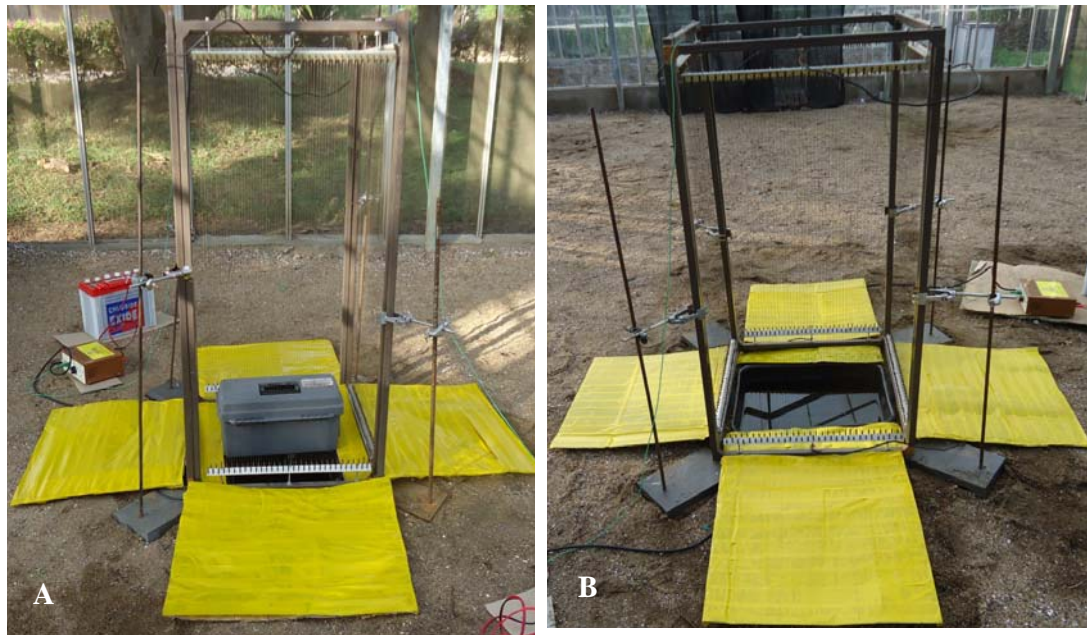
Figure 15: Set up of the fully operating Box gravid trap (A) and the open pond (B) surrounded by a square of electrocuting nets
