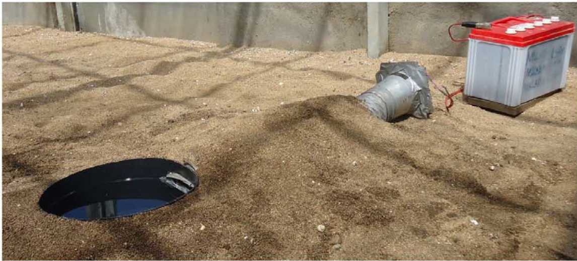
Figure 5. The OviART gravid trap set up. Trap was set by sinking the water-filled bucket into the ground so that the lip of the bucket was flush with the sand surface. The suction tube was buried in the sand leaving only the end with the fan exposed above the soil in order to let airflow freely.
