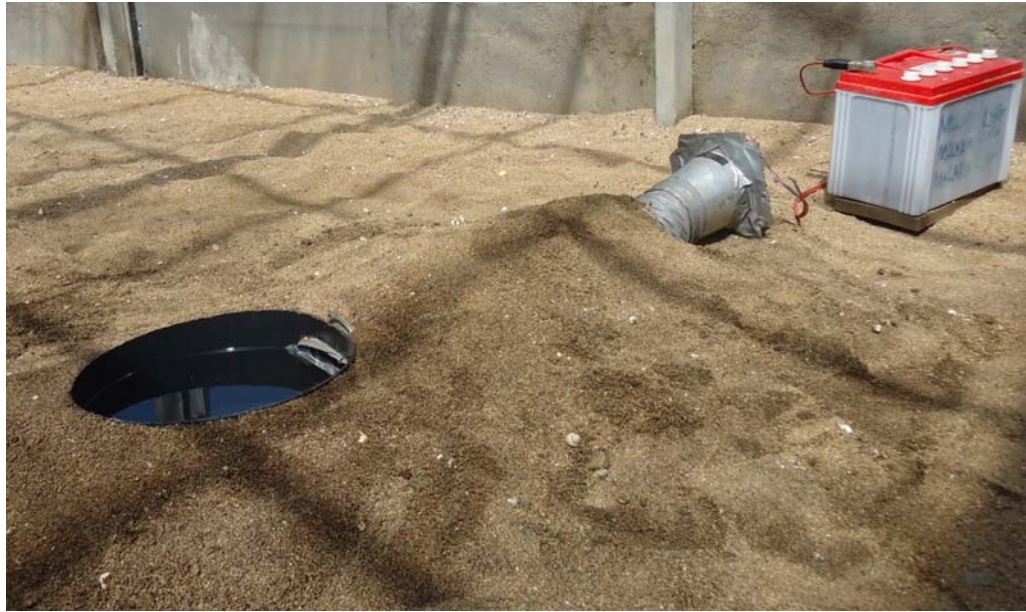
Figure 17: The OviART gravid trap set up, A) the sedge of the bucket at the level of sand B) Water level and inlet of the suction duct
