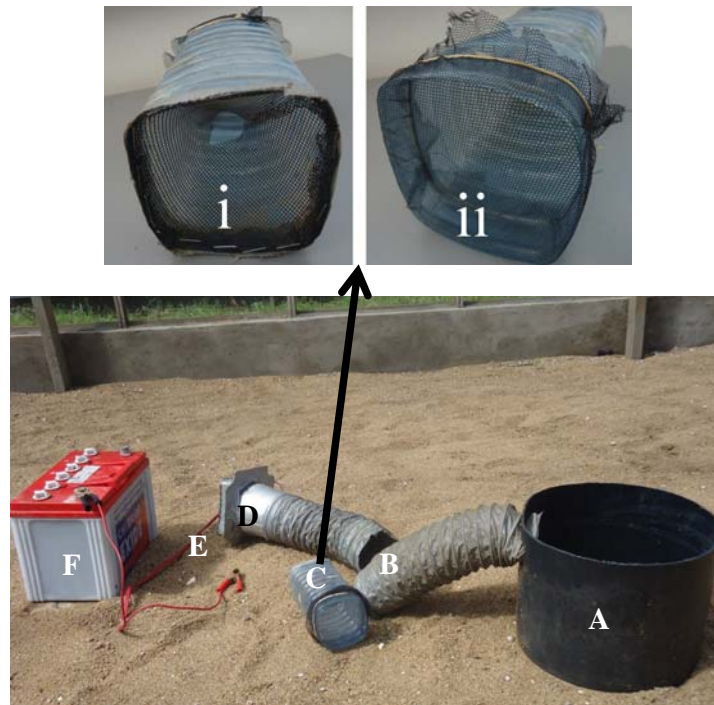
Figure 16: Ovi-ART gravid trap prototype: A) Round black bucket B) Suction tube prepared from collapsible plastic pipe C) Collection chamber (i. conical net at inlet side ii. removable net at outlet side) D) Fan (12 V, 0.38 A) E) Electric cable F) 12 V battery
