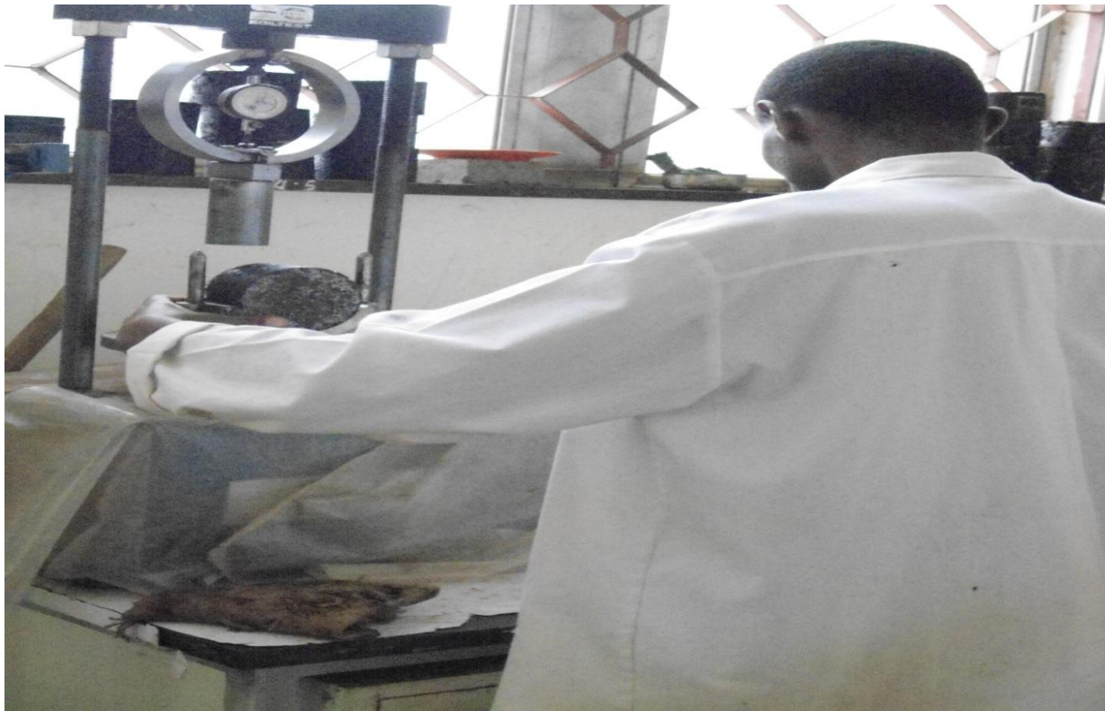
Plate 4.4; A sample being prepared for crushing using Marshall Apparatus during mix design
