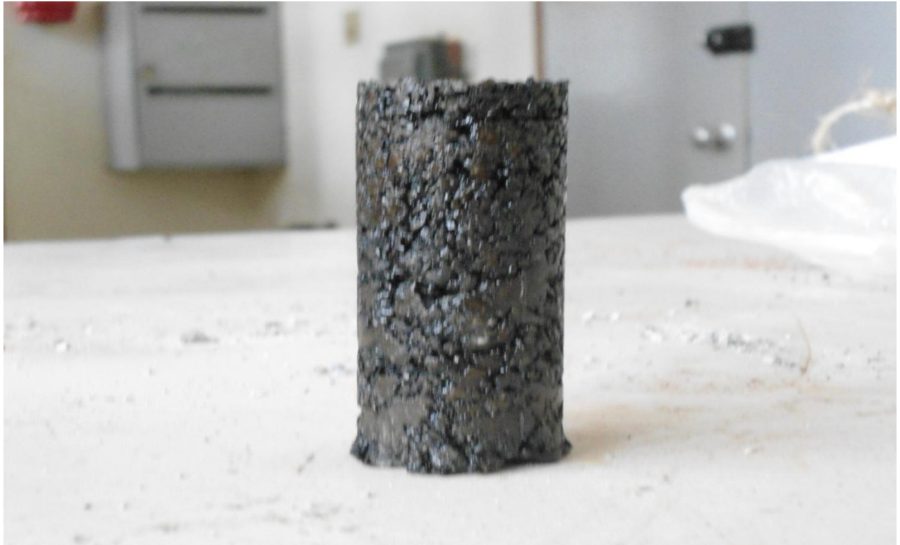
Plate 4.6; Prepared asphalt concrete sample ready for testing by use of triaxial machine
