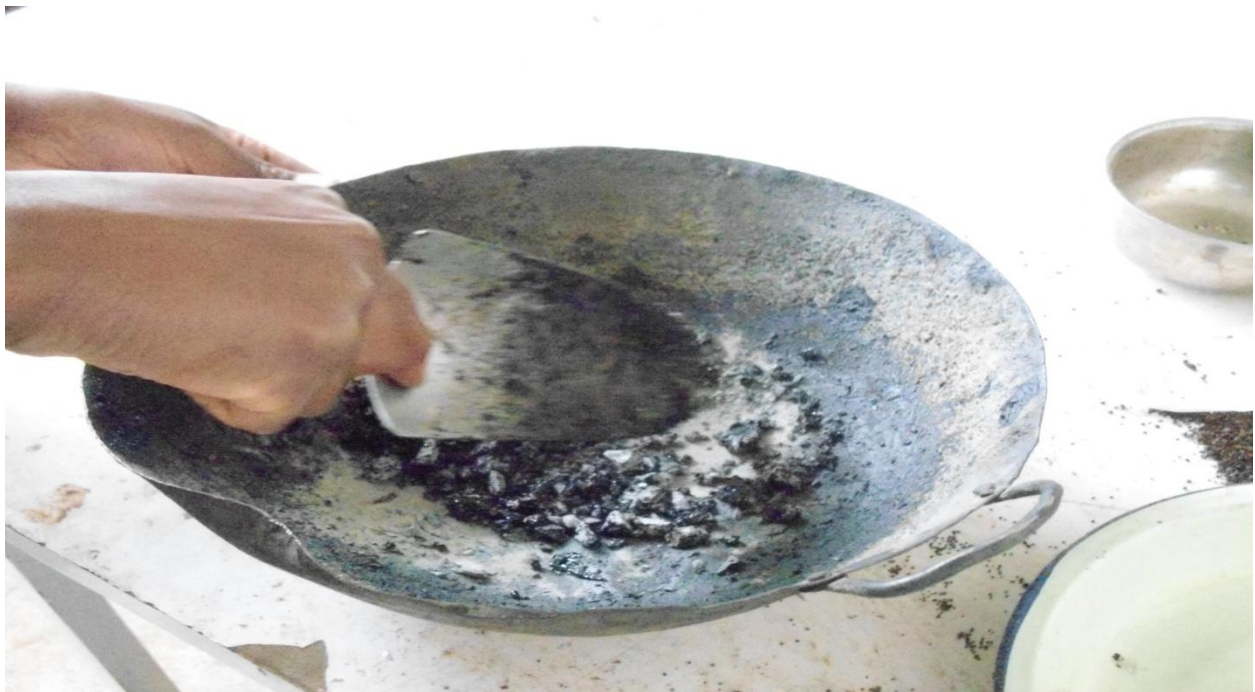
Plate 4.7; Mixing bituminous materials for preparation of asphalt mixture samples to be tested using triaxial compression test
