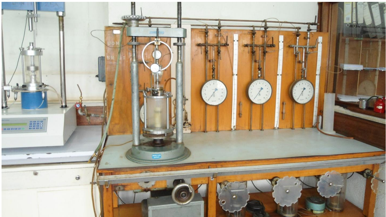
Plate 4.5; Digital triaxial test machine (upper photo) and the manual triaxial test machine (lower photo) at the University of Nairobi soils laboratory.
