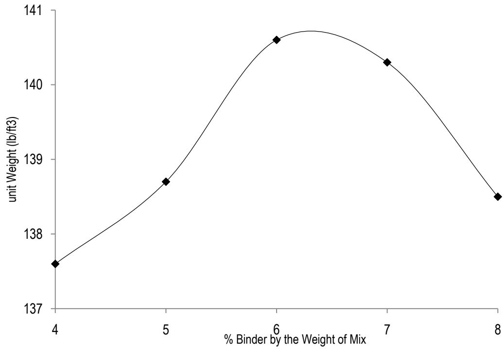
Figure 1.2.1 ; Unit Weight of the Mix Vs % Bitumen Content
