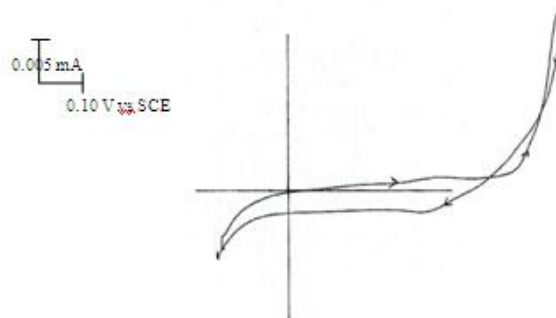
Figure 13: First scan response of polypyrrole in 1.0 M H_2SO_4 . Potential range - 0.2 to 0.80 V, scan rate 20 mV/s.
