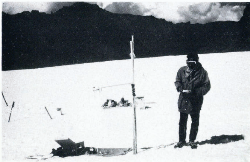
Fig. 2. Installation for measurement of radiation on a vertical surface.
