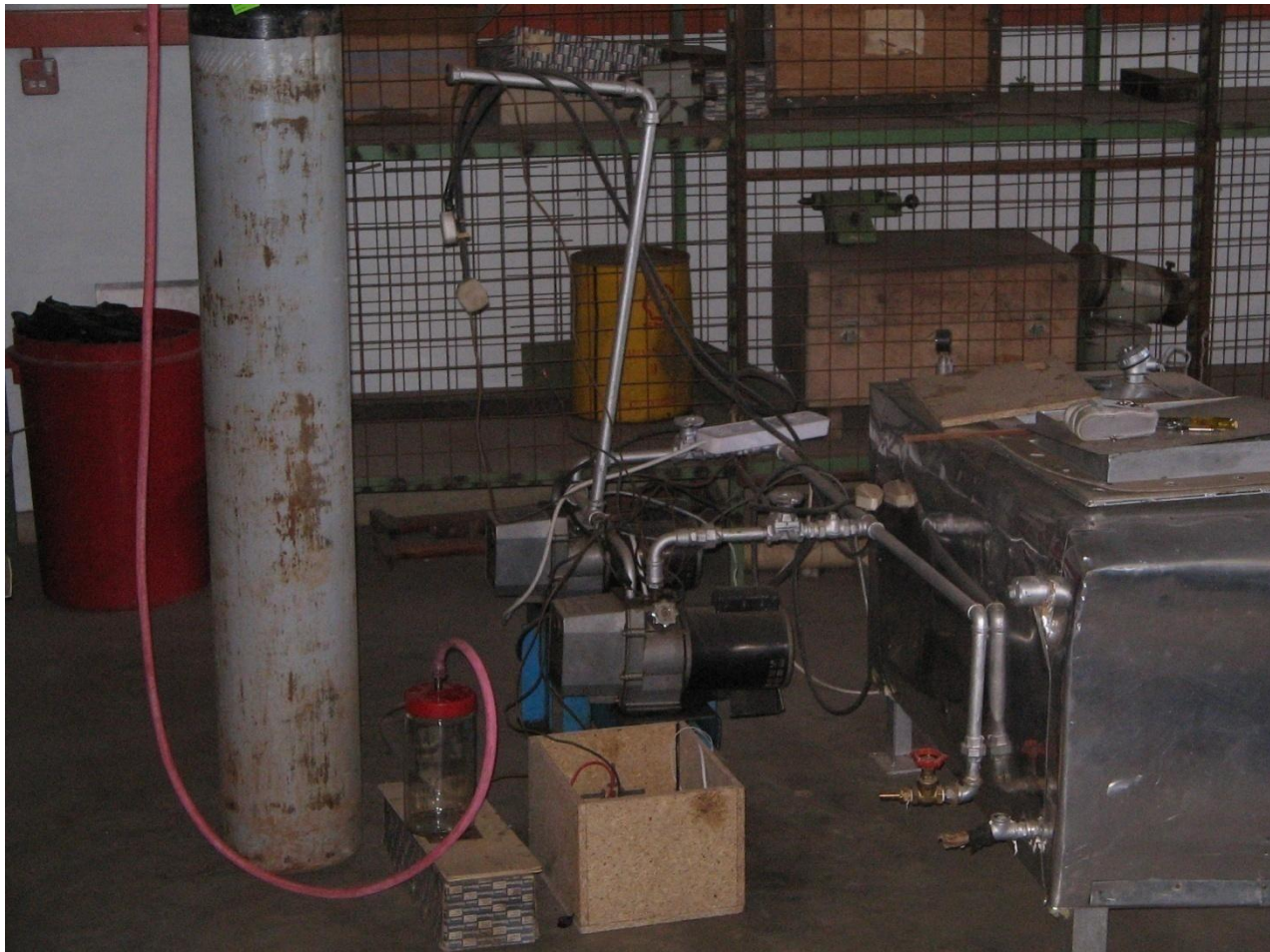
Photo 1: Picture of nitrogen gas, plasma source and Dielectric Barrier discharge chamber
