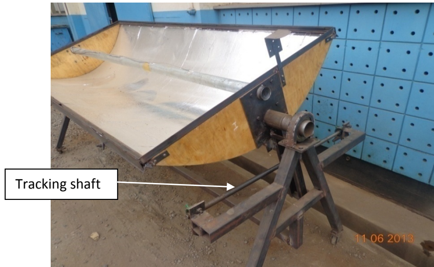
Figure 4.4: The tracking shaft on the concentrator
