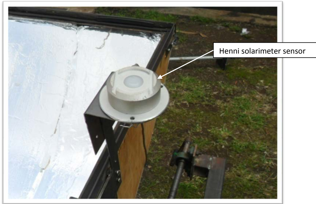
Figure 4.9: Henni solarimeter sensor attached to the trough
