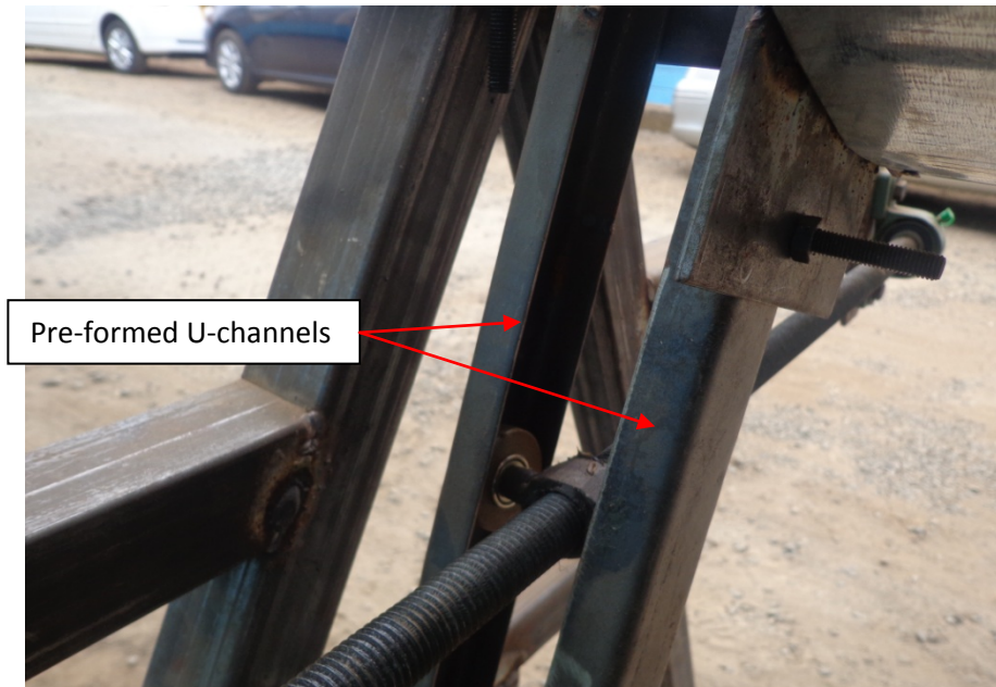
Figure 4.5: Tracking system on the concentrator
