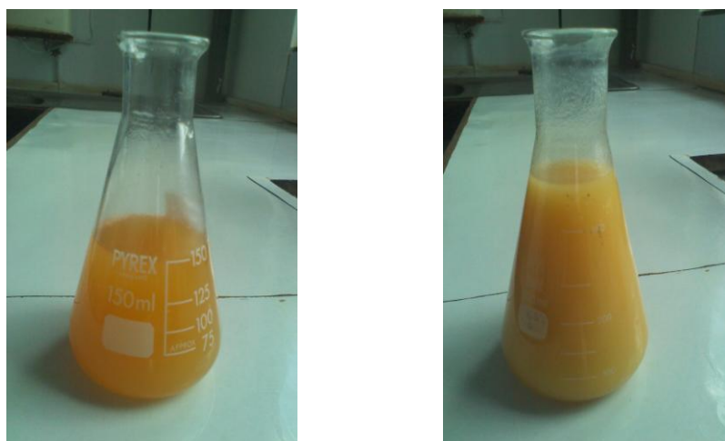
Fig. 3.2: Molten Nile perch ( Lates niloticus ) viscera oil. Crude (left) and high melting point (right) fractions
