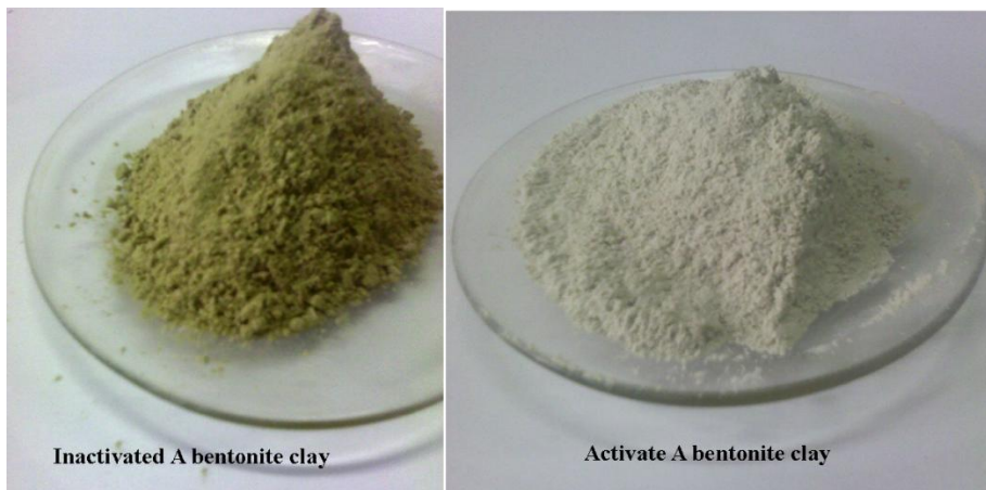
Figure 4.9: Raw (inactivated-left) and activated (right) A bentonite clays
