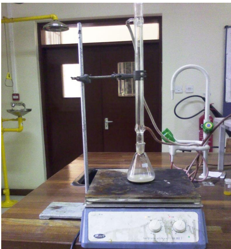
Figure 3.1: Set up of acid activation process
