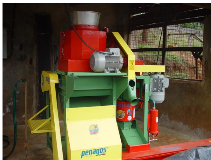
Figure 2.6: A coffee pulper with an inbuilt demucilager
