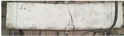
6.3: Failure pattern of L.B. 741
