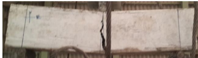
6.7: Failure pattern of Steel 101
