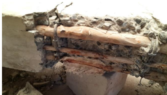
Figure 9: Unsnapped L.buchananii tensile reinforcement
