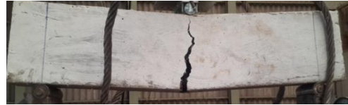
6.4: Failure pattern of L.B. 710
