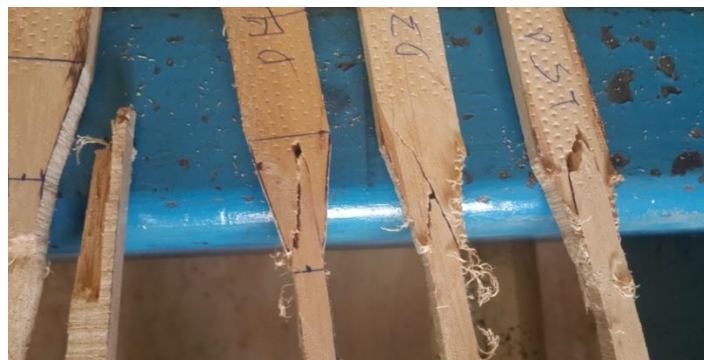
Figure 4: Mode of failure of tensile test samples
