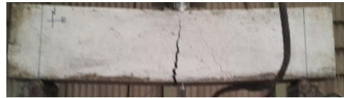
6.2: Failure pattern of L.B. 787
