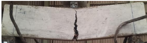
6.5: Failure pattern of L.B. 419
