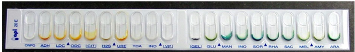
Figure 4.1b. Uninoculated strip of api 20E consisting of 20 microtubes containing dehydrated substrates for the demonstration of enzymatic activity or the fermentation of carbohydrates.
