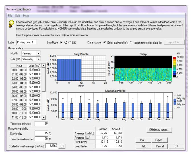
The software then calculated the peak primary load and found it to be 10MW.
