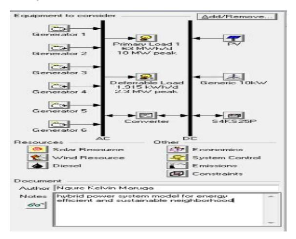
The primary load was calculated by using the same formula used to calculate the maximum demand. This primary load is load that has to be satisfied throughout the day and in this case it was the sum of lighting load and small power load.
