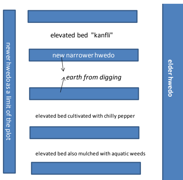
Figure 1: New adjustments in hwedo through a net of perpendicular smaller channels and elevated beds
