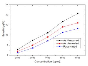
Figure 13. Sensitivity versus CO<sub>2</sub> concentration (ppm).
