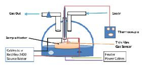
Figure 4. Lab Assembled Gas Sensing Unit
