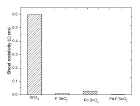
**Figure 8.** Sheet resistivity characteristics of SnO<sub>2</sub>, F:SnO<sub>2</sub>, Pd:SnO<sub>2</sub> and Pd-F:SnO<sub>2</sub> thin films
