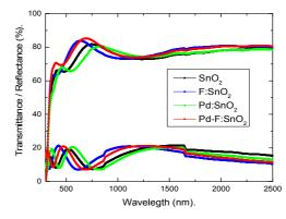
Figure 5. Transmittance and reflectance spectra for doped SnO<sub>2</sub> thin films
