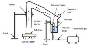
Figure 1. Spray pyrolysis experimental set up.
