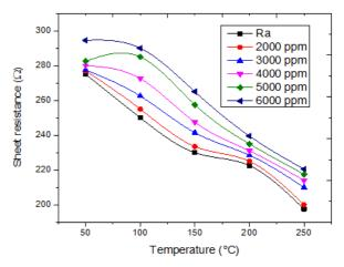
*Figure 11.* Sheet resistance versus temperature for the as annealed Pd-F:SnO<sub>2</sub> thin film.
