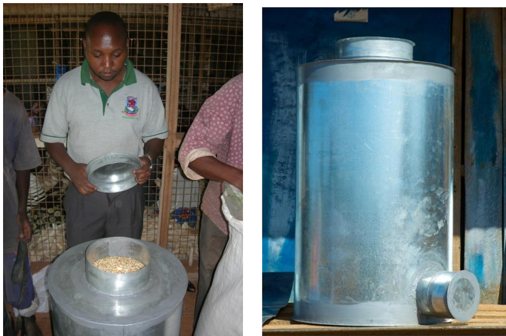
Figure 9: Metal grain silos for small scale storage
