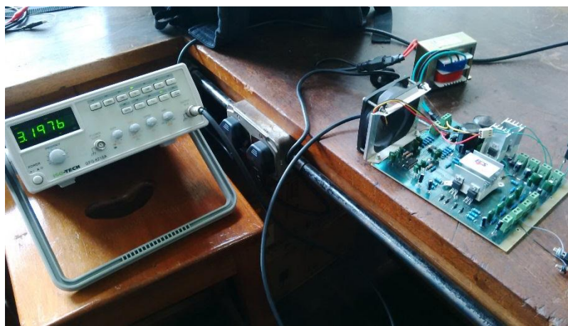
Figure 43: Signal Input connected to a Signal Generator
