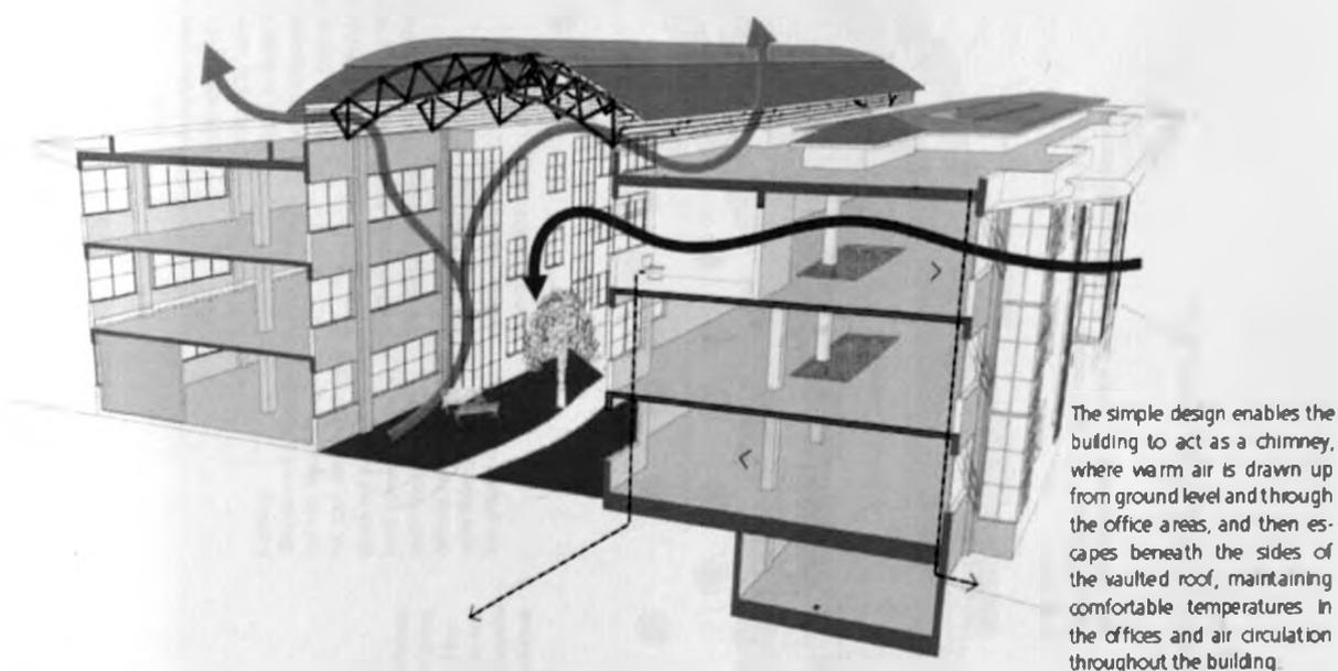
Figure 2.2: Environmental Features of the Building at a Glance
