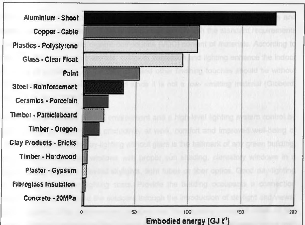
Figure 2.1: A graph showing embodied energy content of selected Building materials
