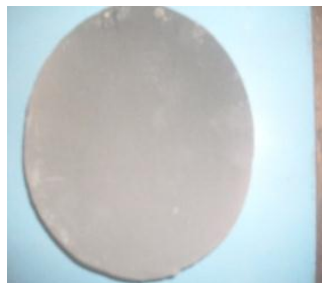
Figure 4.2a: Poorly fired disk ceramic filter
