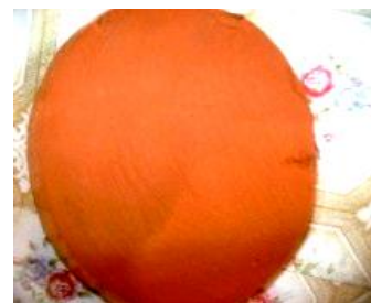
Figure 4.2b: Optimal fired disk filter at 950°C
