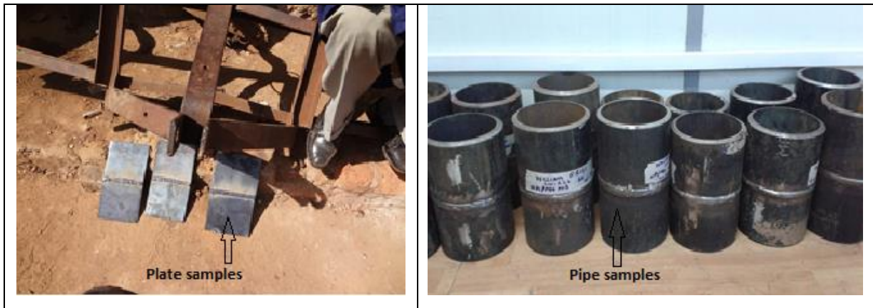
Figure 3.1: Plate and pipe test coupons analyzed
