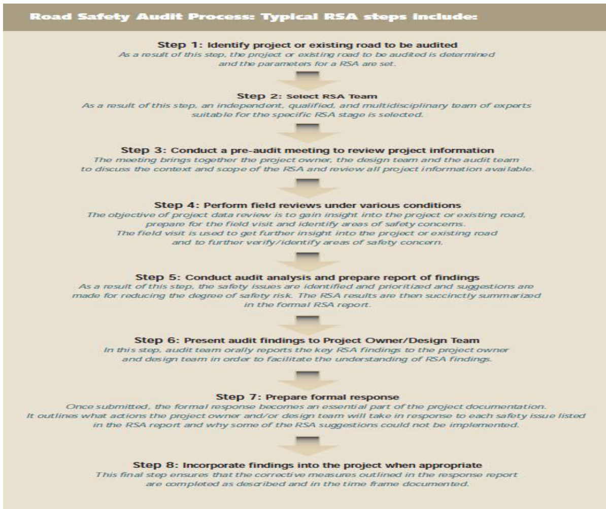
Figure 2.9 The typical eight-step RSA procedure
