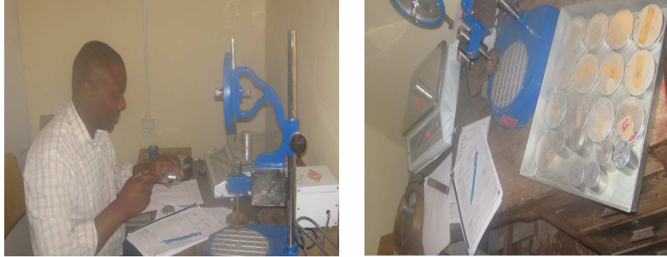
Plate 3.1 Testing of soil liquid limit using Cone penetrometer (Left) Determining soil moisture content (Right).
