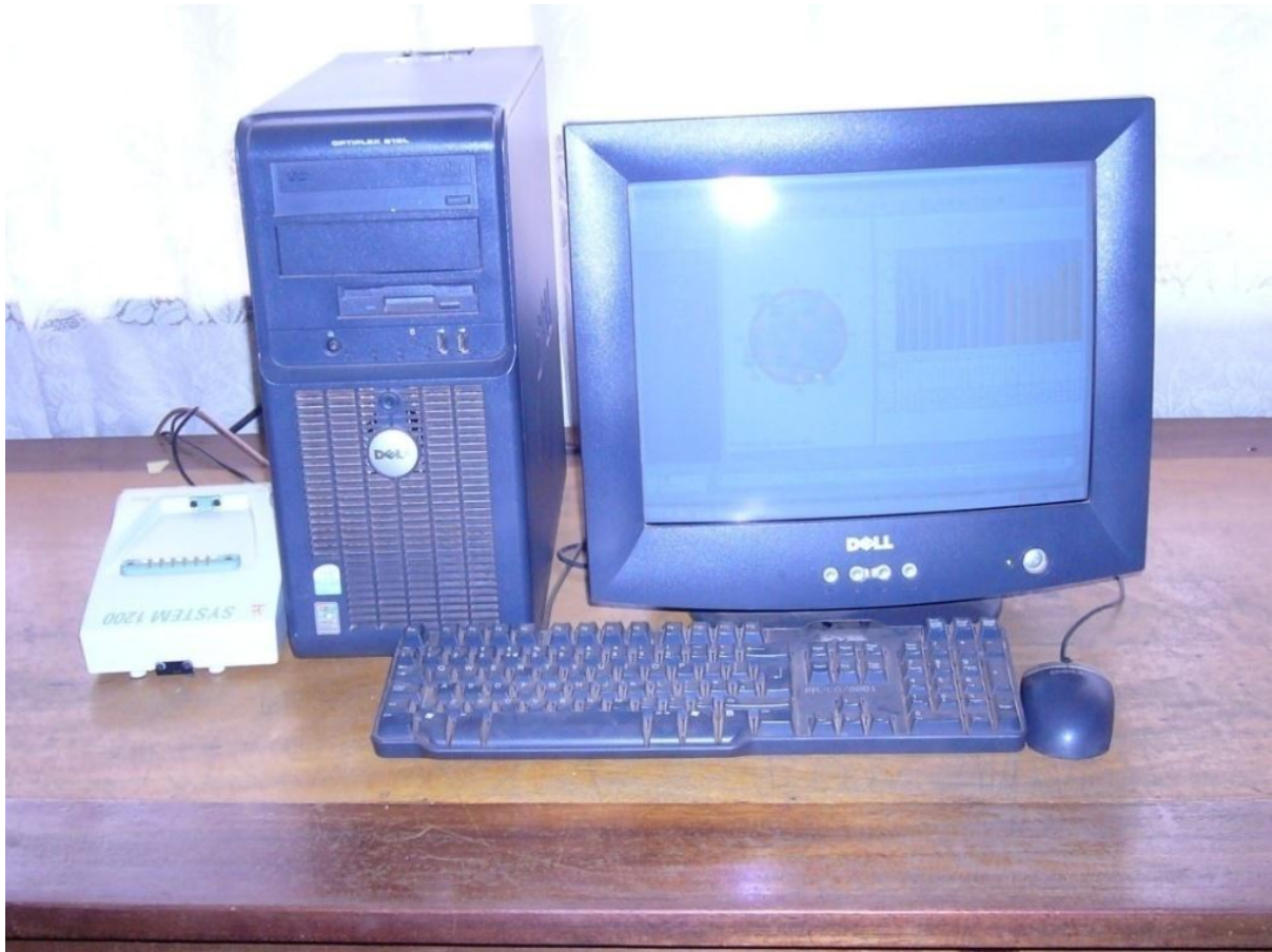
Figure 4-2: GPS Receiver Setup at RCMRD including receiver on the left and computer for data processing.
