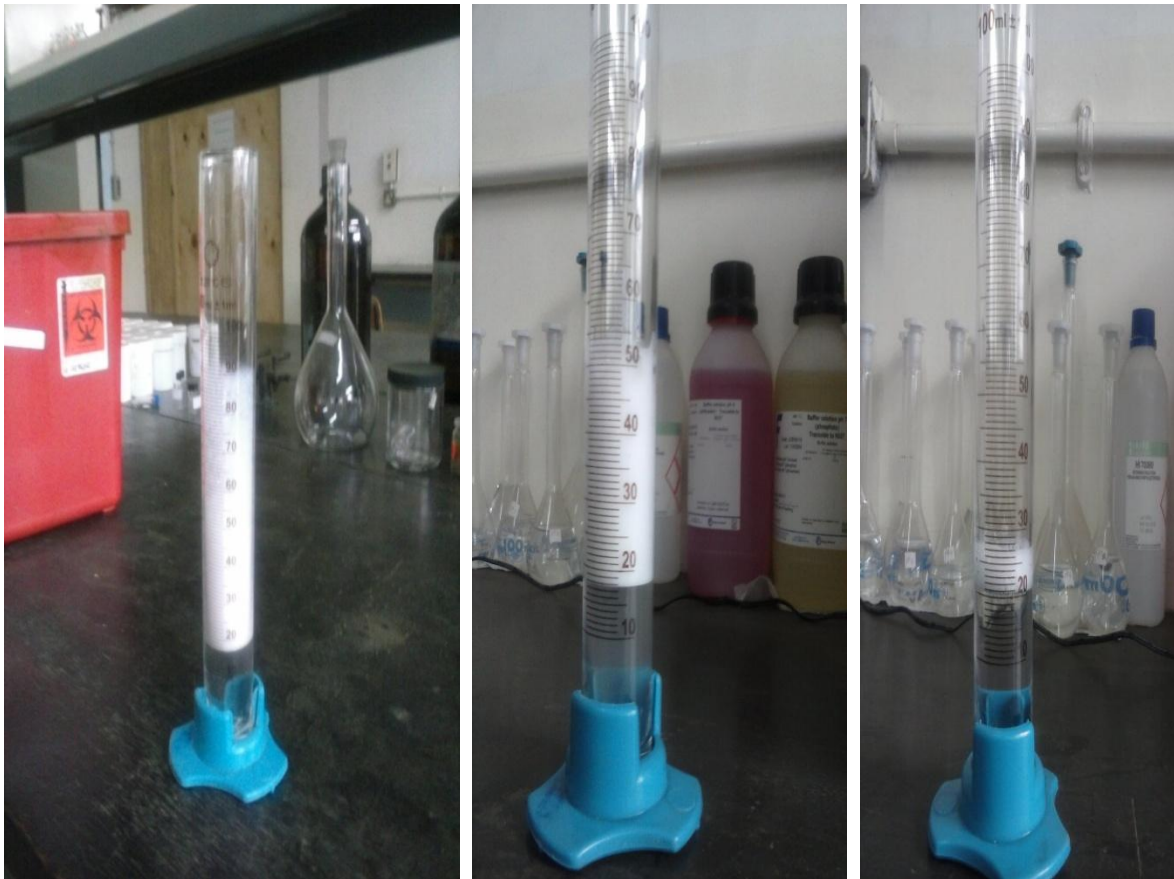
Figure 4.5: Foam height of the ethanol extract, raw gum and the water extract respectively.
