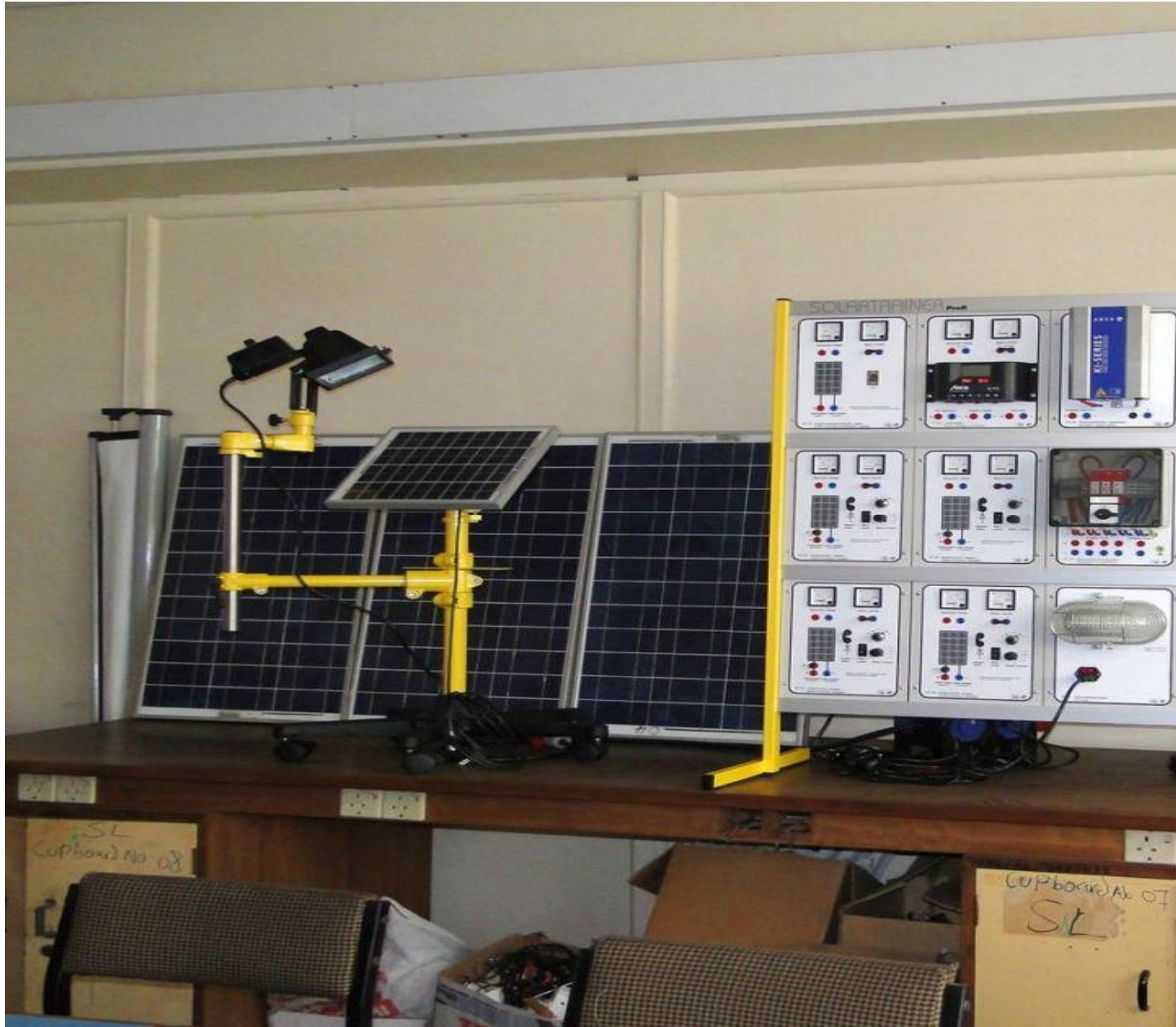
The solar trainer KIT for advanced PV training in grid-tie and hybrid systems
